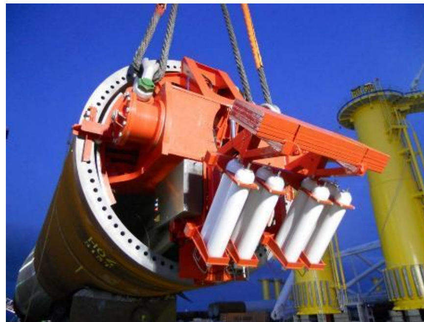
Figure 50 Monopile upending tool, courtesy of Houlder.
