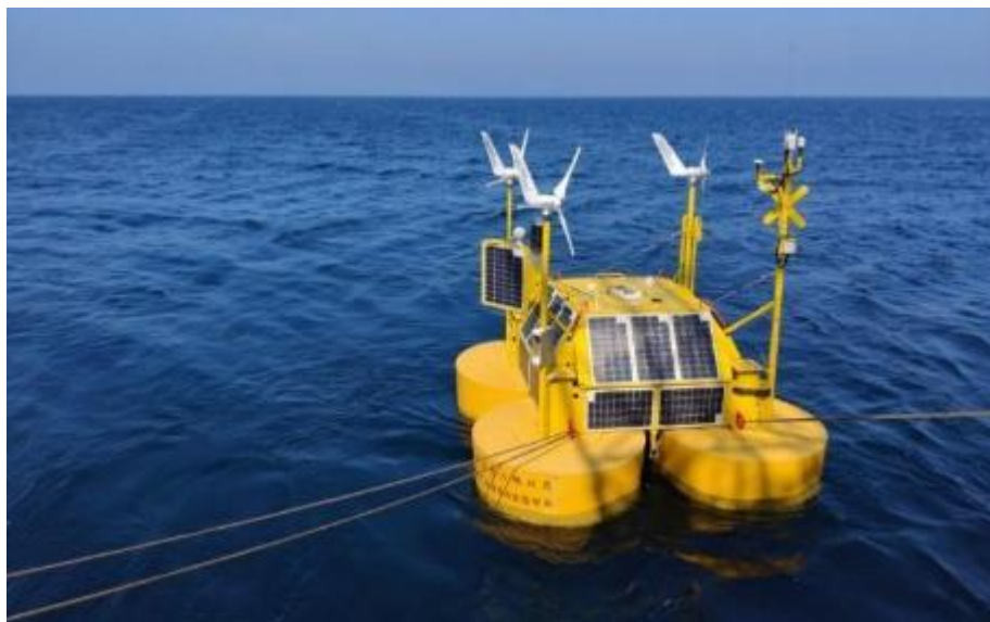
Figure 7 Example of a floating lidar used to capture atmospheric data. Image courtesy of EOLOS. All rights reserved.
