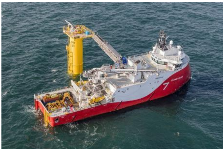
Figure 62 Installation support vessel carrying out electrical termination and testing works, courtesy of Subsea7.
