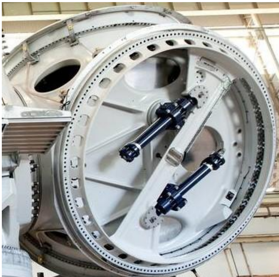
Figure 24 Hub casting (shown assembled with pitch system and blade bearings), © Vestas.
