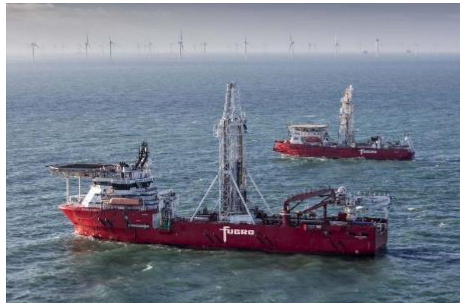
Figure 10 Geotechnical survey and drilling vessels Fugro Synergy (front) and Fugro Bucentaur (back), courtesy of Fugro.
