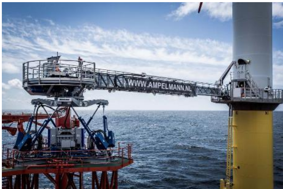
Figure 73 Full motion-compensated turbine access system, courtesy of Ampelmann.
