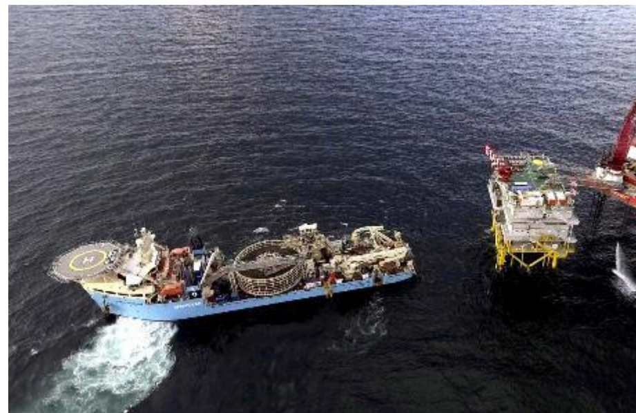
Figure 57 Cable-laying vessel Maersk Connector, courtesy of DeepOcean.
