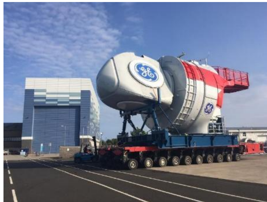
Figure 12 GE's Haliade X 12 MW nacelle. Image courtesy of GE VernovaRenewable Energy. All rights reserved.
