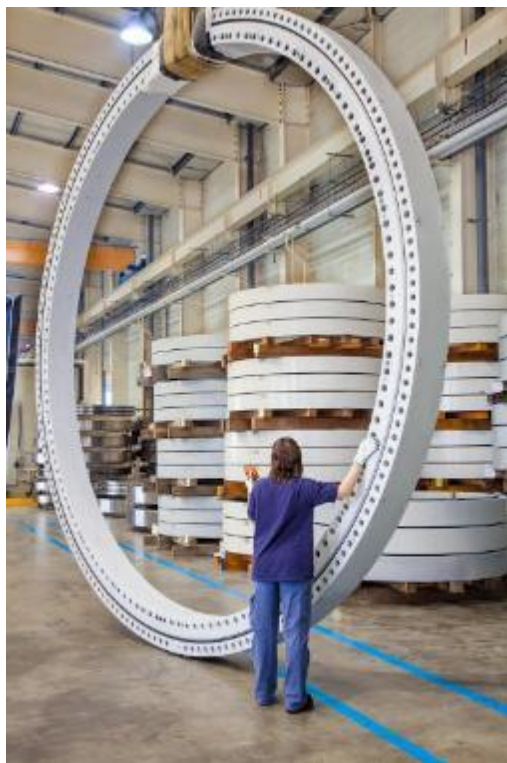
Figure 25 Blade bearings, courtesy of Rollix.
