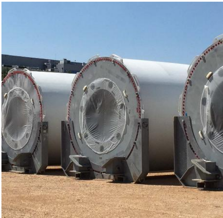
Figure 23 Wind turbine blade roots, courtesy of GE Vernova.
