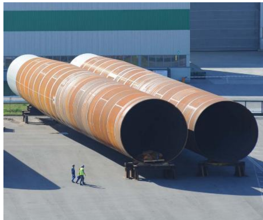
Figure 34 Monopile foundations, courtesy of EEW SPC, © Andreas Duerst, STUDIO 301.
