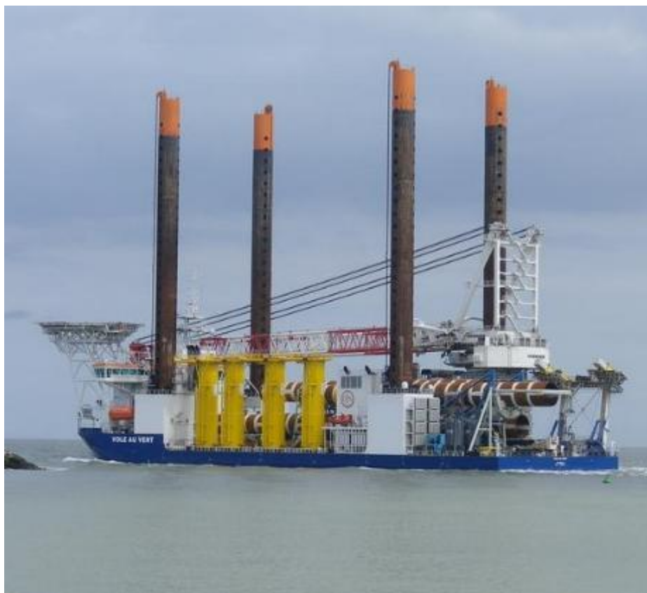
Figure 49 Foundation installation vessel, courtesy of Jan de Nul.
