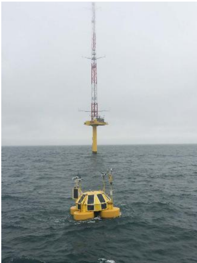
Figure 69 Floating lidar, courtesy of EOLOS Floating Lidar Solutions.
