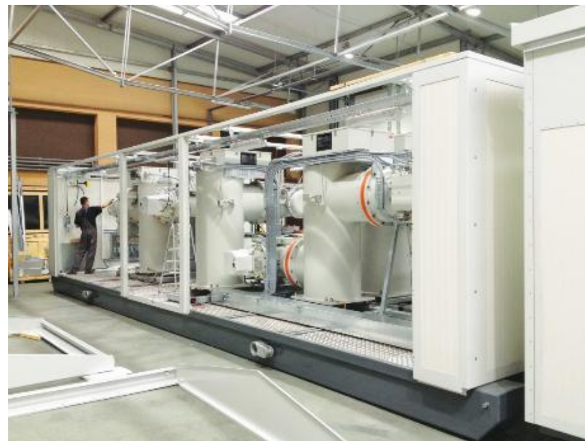
Figure 44 Gas-insulated switchgear, © ABB.
